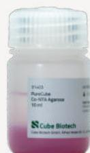
Co-NTA can significantly increase protein purity during purification. However, its binding capacity is reduced when compared to Ni-NTA. Binding Capacity: 40 mg/ml as Agarose and 30 mg/ml as MagBeads. Which is still far above other affinity tags.
