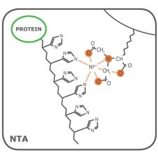
Fig. 1: IMAC chelating ligands IDA and NTA. Iminodiacetic acid (IDA) and nitrilotriacetic acid (NTA) are widely used to fix transition metal ions to a matrix, which then serves as an affinity resin. The two ligands differ in the number of valencies with which they coordinate the metal ion (IDA is trivalent, whereas NTA is tetravalent; valencies highlighted in orange), which impacts the quality of the purified protein fraction.
